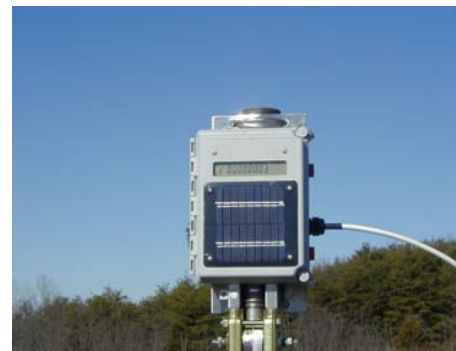
Chart Replacement with 1-Watt Solar Panel
